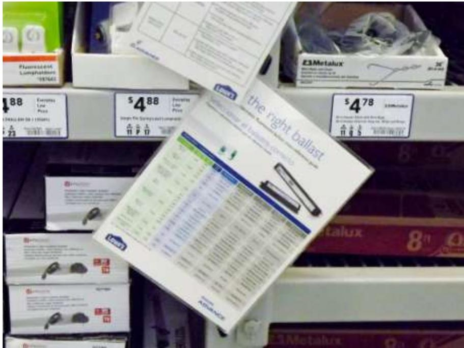
**Figure 1.4 – This info sheet provides a cross reference for electronic ballasts when replacing older magnetic ballasts. It does not provide any information on the FCC rules pertaining to Part 18.**
