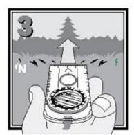
Read the bearing at the compasses index line, and follow the bearing in the field.
