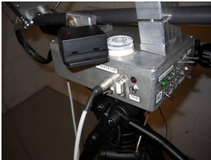
Fig 11 Control Box with GPS unit (Black Box)
