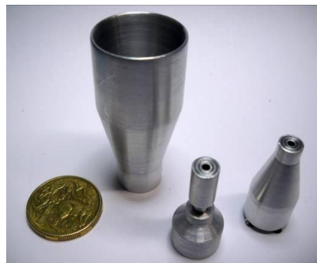
Fig 9 Horn, Adjustable and fixed feeds
