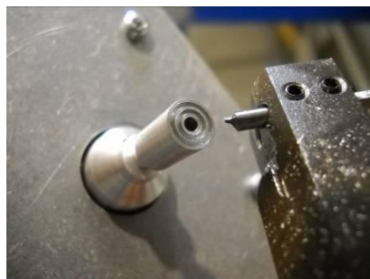
Fig 8 Tiny Multi Choke Ring dish feed Commonly known as Chaparral TM (The centre hole is 5/64" Diameter)
