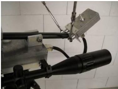
Fig 10 Feed point and Telescopic sight
