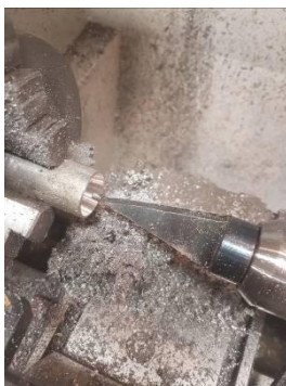
Fig 7 Horn boring
