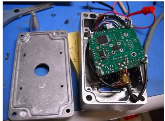
Fig 14 Inside the dish feed box
