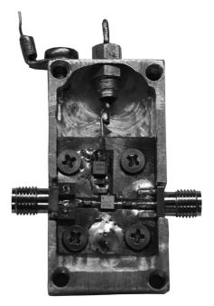
Figure 6 — Assembled prescaler in a machined aluminum housing.
