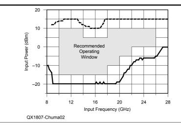
Figure 2 — Input sensitivity window of the HMC447LC3.
