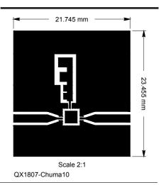
Figure 10 — PCB layout of the multiplier.
