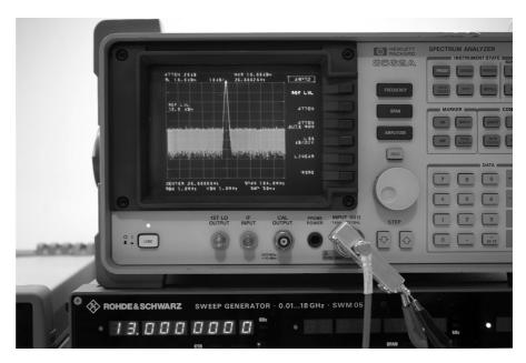
Figure 12 — Testing the multiplier shows13 GHz input and 26 GHz output signals.
