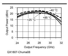
Figure 8 — Output power vs. frequency and temperature with +4 dBm drive level to the HMC942LP4E.
