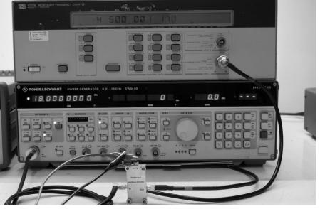
Figure 7 — Testing the prescaler with 18 GHz input and 4.5 GHz output signals.
