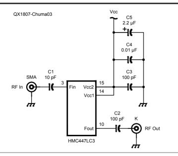
Figure 3 — Schematic circuit of the prescaler using the HMC447LC3. The package base is ground.
