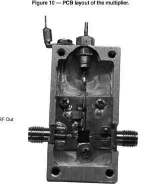
Figure 11 — Assembled multiplier/doubler in a machined aluminum housing.
