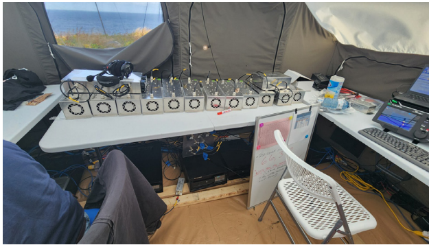
A diplexer, a triplexer, and band-pass filters in use at the CY9C St. Paul DXpedition. [Glenn Johnson, WØGJ, photo]
