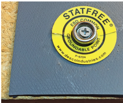
Figure 3 — The antistatic mat ground connection point.
