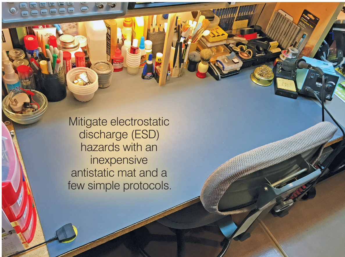
Figure 1 — A large antistatic mat covering the author's workbench. The mat's ground connection is at the lower left, which also provides a wrist strap connection point.
