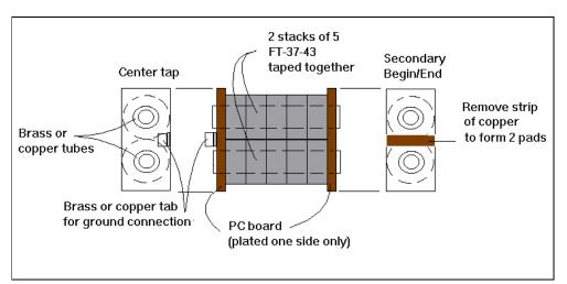
flashing copper to form the center tap. Be sure to leave a tab on the center tap for connecting to the circuit board. Make two similar tabs for the secondary connections on the other end of the cores. Wind three complete turns through both cores with Teflon insulated AWG #22 stranded wire. The wire ends should extend out of the core end with the center tapped secondary.
