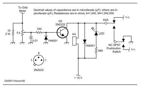
Fig 13—Schematic of optional grid circuit protection scheme. K4 is a DPDT 12 V dc relay
