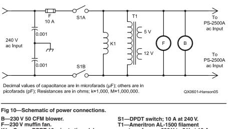
F—230 V muffin fan. K1—Omron DPDT 10 minute time delay relay.
