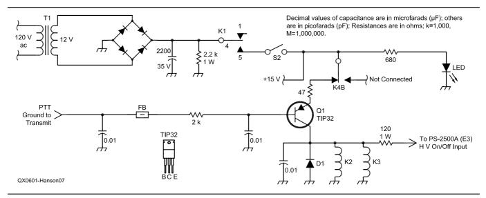
Fig 12—Schematic of control wiring. K2 and K3 are Schrack SPDT 12 V dc relays.
