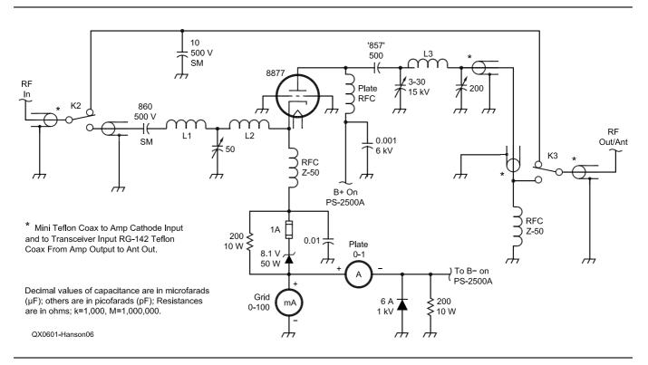
Fig 11—RF deck schematic. L1 and L2 are 9 turns 16 gauge, 1/2 inch diameter by 1 inch long. L3 is 4 turns, 3/16 inch tubing, silver plated 11/2 inch diameter by 3 inches long. The plate RFC is 12 turns 20 gauge Formvar close wound on a 1/2 inch teflon rod. The filament choke is 10 turns 14 gauge formvar each, bifilar wound on a 1/2 by 2 inch ferrite rod.
