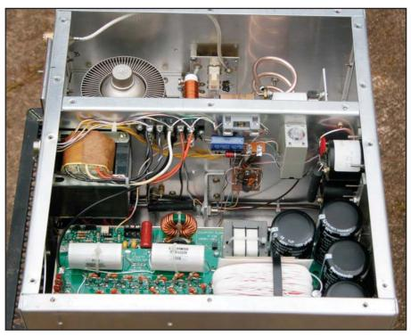
Fig 6—Another view of RF deck, showing the 8877, anode clamp and input/output relayswitching board, featuring the Schrack relays. Also note the Teflon RG-142 coax for the output. This coax will handle the 1.5 kW without meltdown! Also shown is part of the control circuitry—the Omron time delay relay and Tripplett 120G series plate and grid meters. The fuse at the center is for the amplifier cathode circuit. The filament/control transformer at the left is an Ameritron 406-1419-3J.
