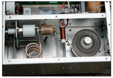
Fig 7—Larger view of the tank circuit, showing the silver-plated tank coil, 3 to 30 pF vacuum variable capacitor, 857 blocking capacitor, RF plate choke and, almost buried at the bottom, the 200 pF loading capacitor.
