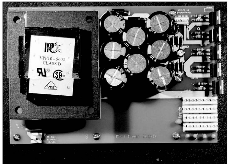
Fig 2—Photo of completed power supply.
